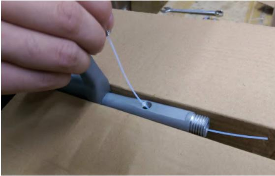
5. Screw the new spare part (C) with the internal hose with wrench size 14 into the housing. Then screw the switching unit in place with wrench size 16 and brace with wrench size 14.
