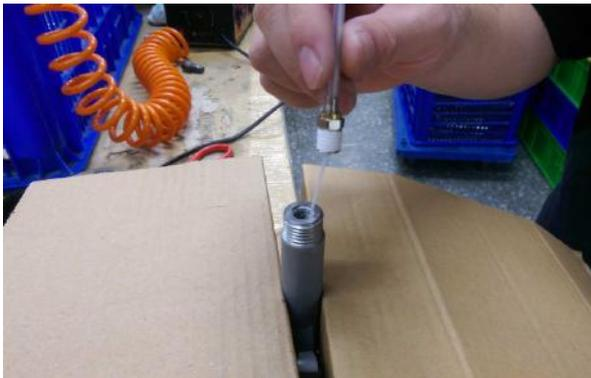
7. Lay the blue Tornador hose (A) over the internal hose (C) and screw it into the housing (B) with wrench size 10.
