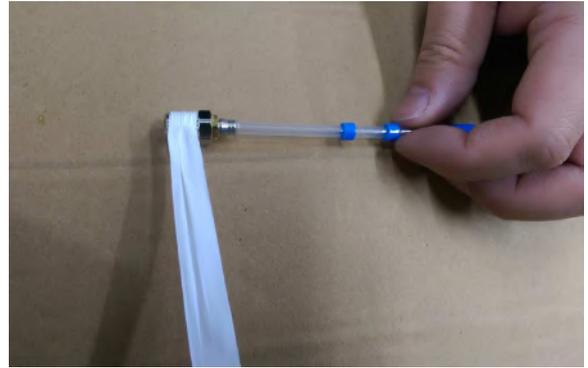
6. Wrap the thread of the blue Tornador hose with sealing tape and remove any protruding ends of sealing tape with a knife.
