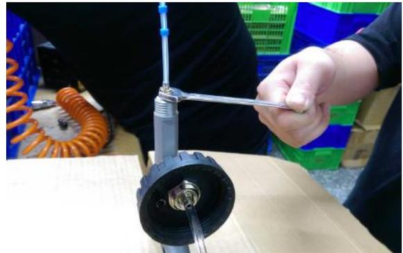
2. Unscrew and remove the screw wrench size 10 with the blue Tornador hose (A) from the housing (B). Remove any residue from the sealing tape from the internal thread of the housing.
