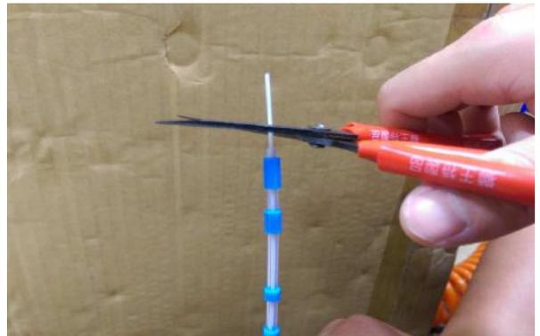
8. Cut off the protruding internal (C) hose so that it is level with the blue Tornador hose (A). Then twist open the spout.
