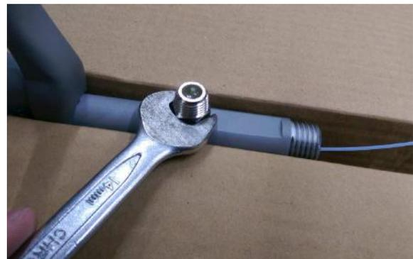
4. Then unscrew and remove the thread with the hose from the housing with wrench size 14.
