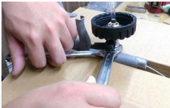
3. Unscrew and remove the size 16 switching unit (D) from size 14 nut (C) above it. Brace with a size 14 open-jaw wrench.
